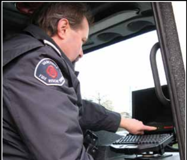
John Wilson, communications trainer for Vancouver firefighters, uses the new i/CAD mobile workstation. Laptops provide firefighters with a GPS location system, direct access to a record management system and real-time updates of events in progress.
